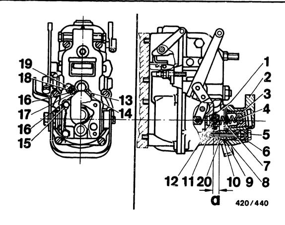
For screwing in and tightening the entire assembly, use is to be made of the modified socket wrench KDEP 2966 (see picture) and the lock nut is to be tightened to 30...35 Nm.
